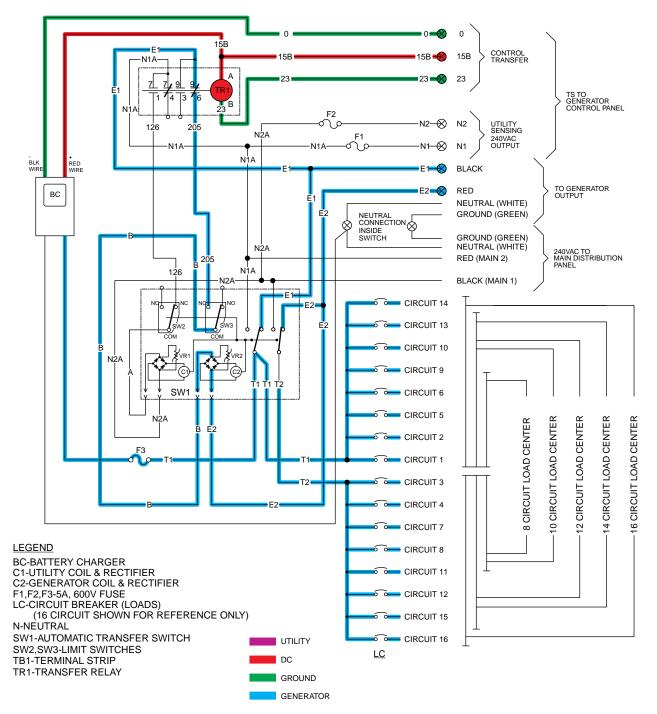
Figure 6. Generator Powering Load.
